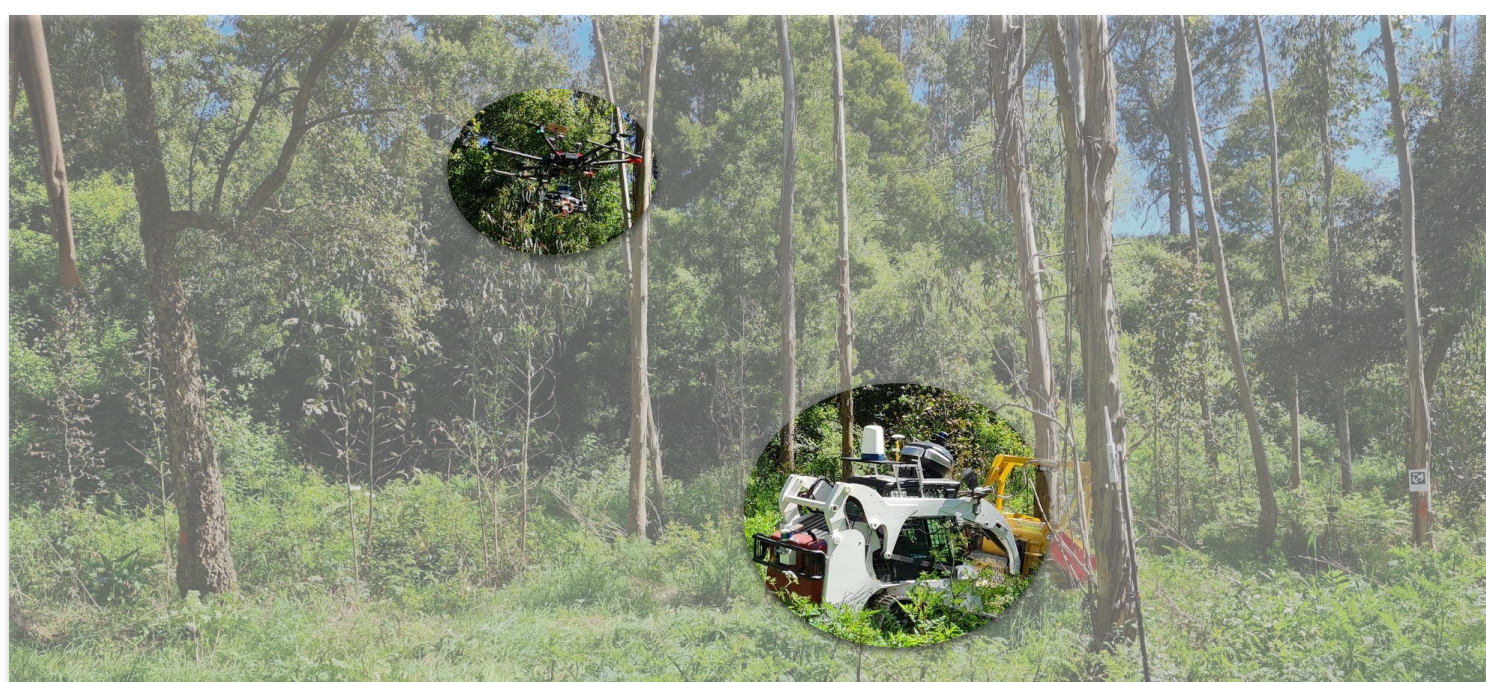
Fig. 1: UAV will generate a mapping of the forest environment and relay information such as locations of flammable vegetation and how traversable a region is to a UGV.
