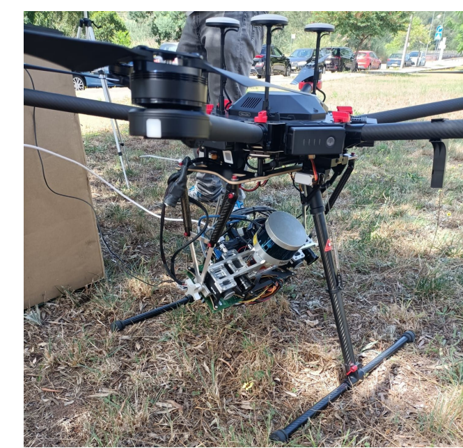
Fig.2. UAV platform with LiDAR payload
